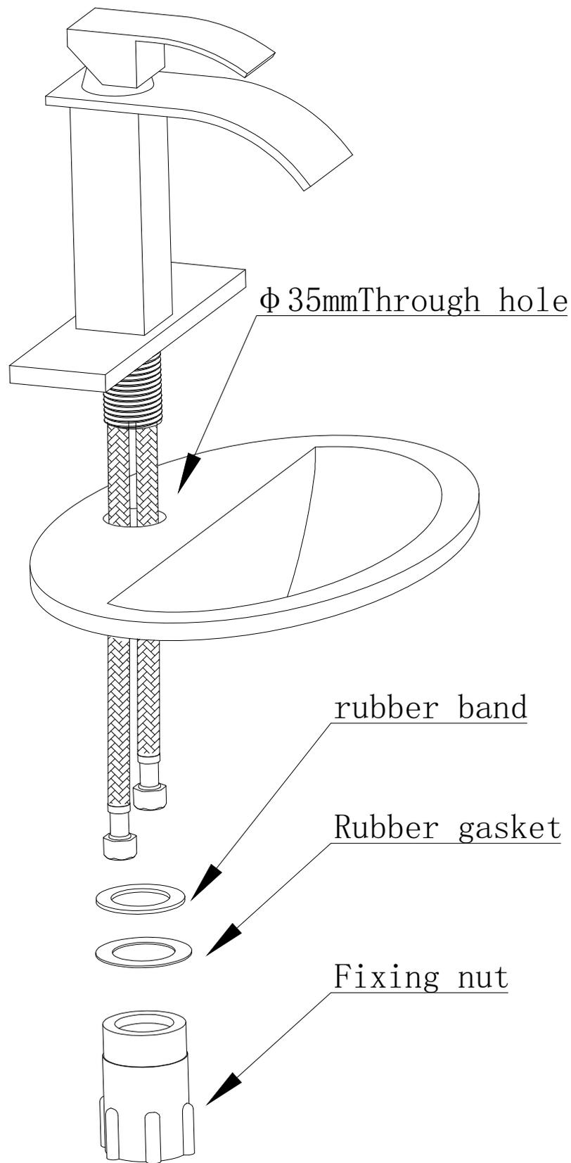
2、 Make sure the basin has a  $\phi 35\text{mm}$  through hole, pass the hose through the hole, pass the rubber ring, rubber washer, and fixing nut into the hose in the order of the drawing, and tighten the fixing nut and the fixing screw to fix the faucet on the basin
