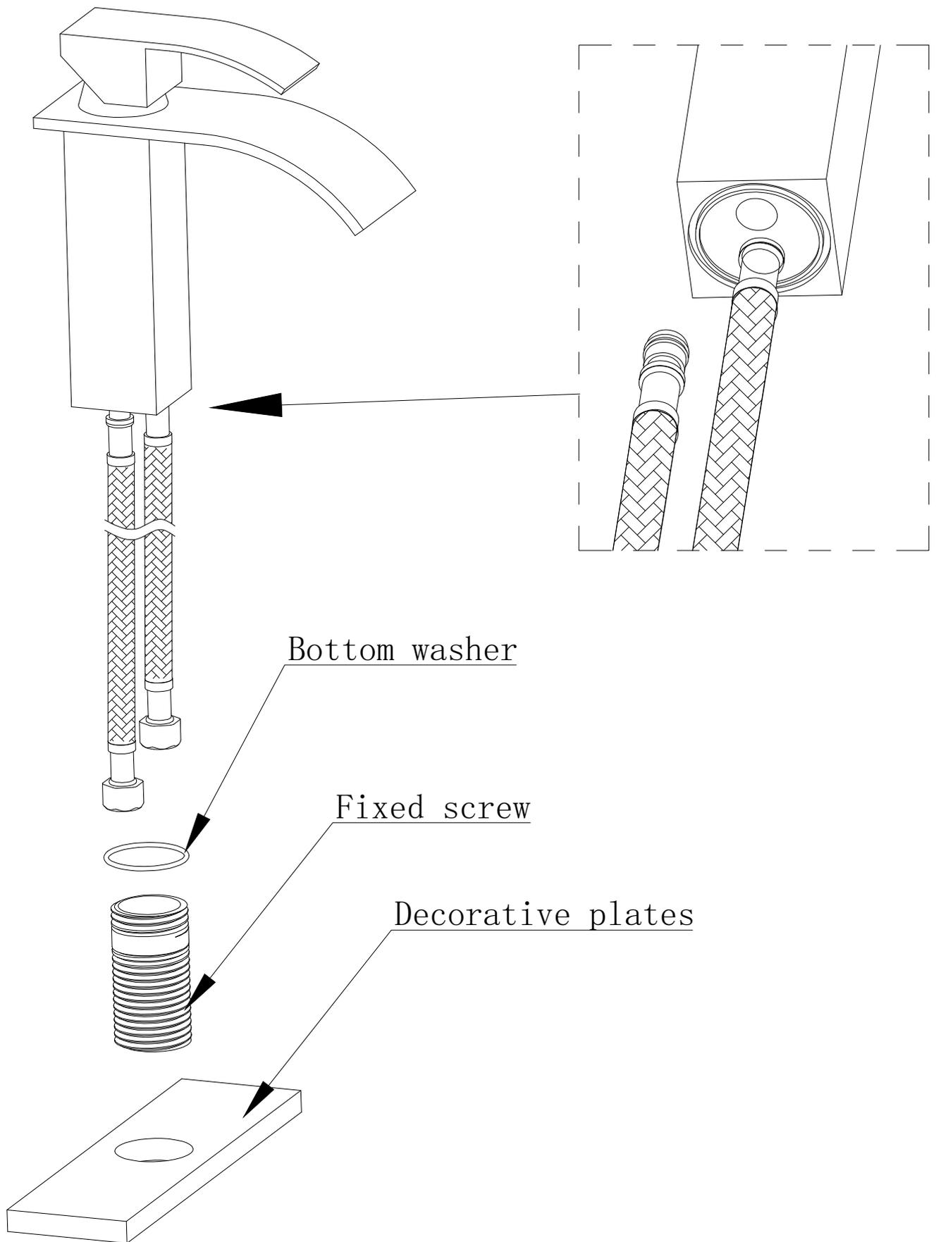
1、 Connect the water inlet pipe to the faucet, then put the bottom gasket into the bottom of the faucet, then tighten the faucet with a fixing screw, and then put on the decorative panel.
