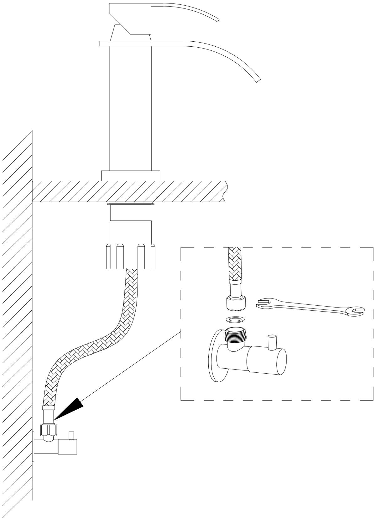
3、 Connect the two inlet pipes on the main body of the faucet to the angle valve. Follow the "red" and "blue" points on the handle of the faucet, the left is red and the right is blue, respectively connecting the "hot"/"cold" water.
